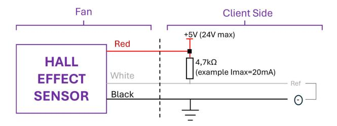
When the motor rotates, the sensor sends a signal to the points Ref and  $\bigcirc$ , with frequency and width Ts proportional to the rotation speed (Ts = 60/n).
